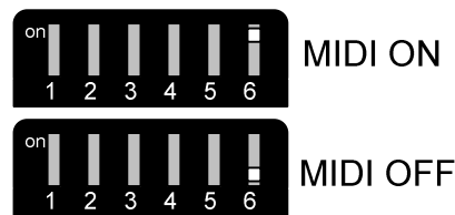
figure 6: Dip-Switch setting for MIDI-Insertion
